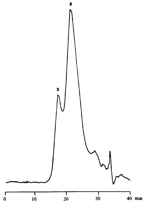
Figure 4 Size-exclusion chromatography of purified 104-mer. Top trace shows tetrameric (labelled 1) and monomeric (labelled 2) forms obtained from the isolation of the material retained on the cationic-exchange column. Bottom trace represent purified peak 2 (Panel A) reinjected on the same column; peak labelled 3 is the dimeric form of 104-mer. Samples were run on a Sephadex 75 column, using buffer containing 20 mM MOPS, 0.5 M NaCl pH 7.0 and a flow rate of 0.5 ml/min. Detection at 280 nm.
